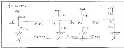
DL on span IJ = 19 KN/m
